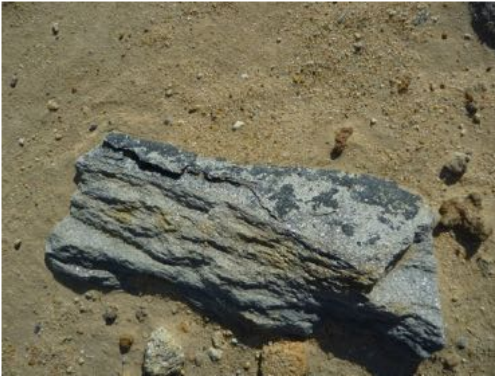
Figure 38 Pyritic sandstone rocks in the mined wetland area
