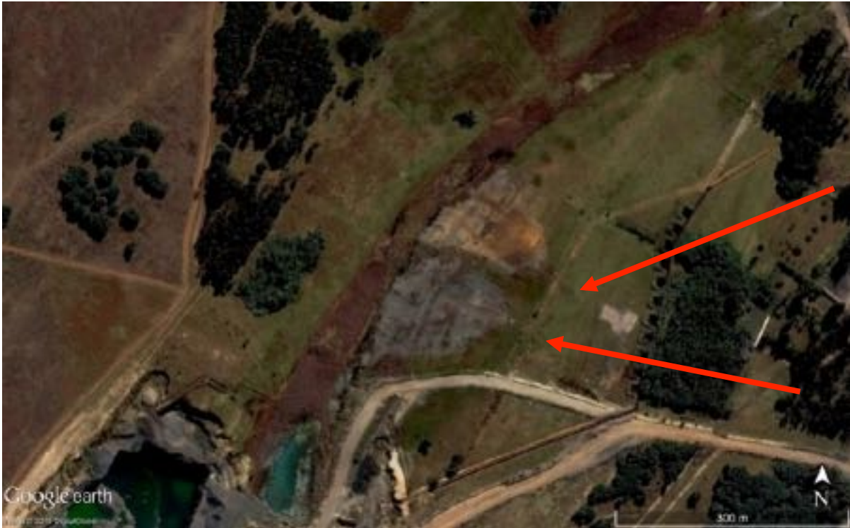
Figure 60 Acid water outflow zone (with visible plume) through boreholes (red arrows) that “punctured” an underground disposal facility
