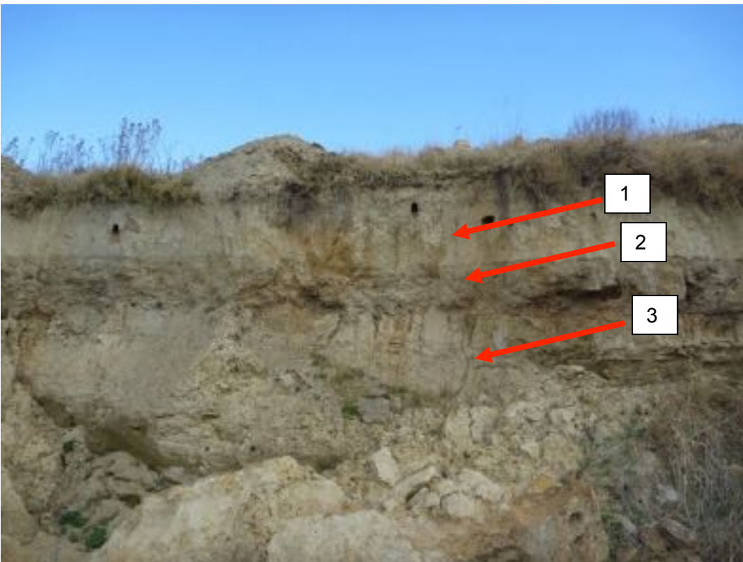
Figure 17 Opencast mine profile indicating 1) a thin bleached soil profile overlying 2) a hard plinthic layer and 3) weathered sandstone
