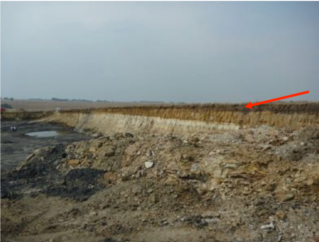
Figure 16 Opencast mine profile indicating a thin bleached soil profile (arrow)
