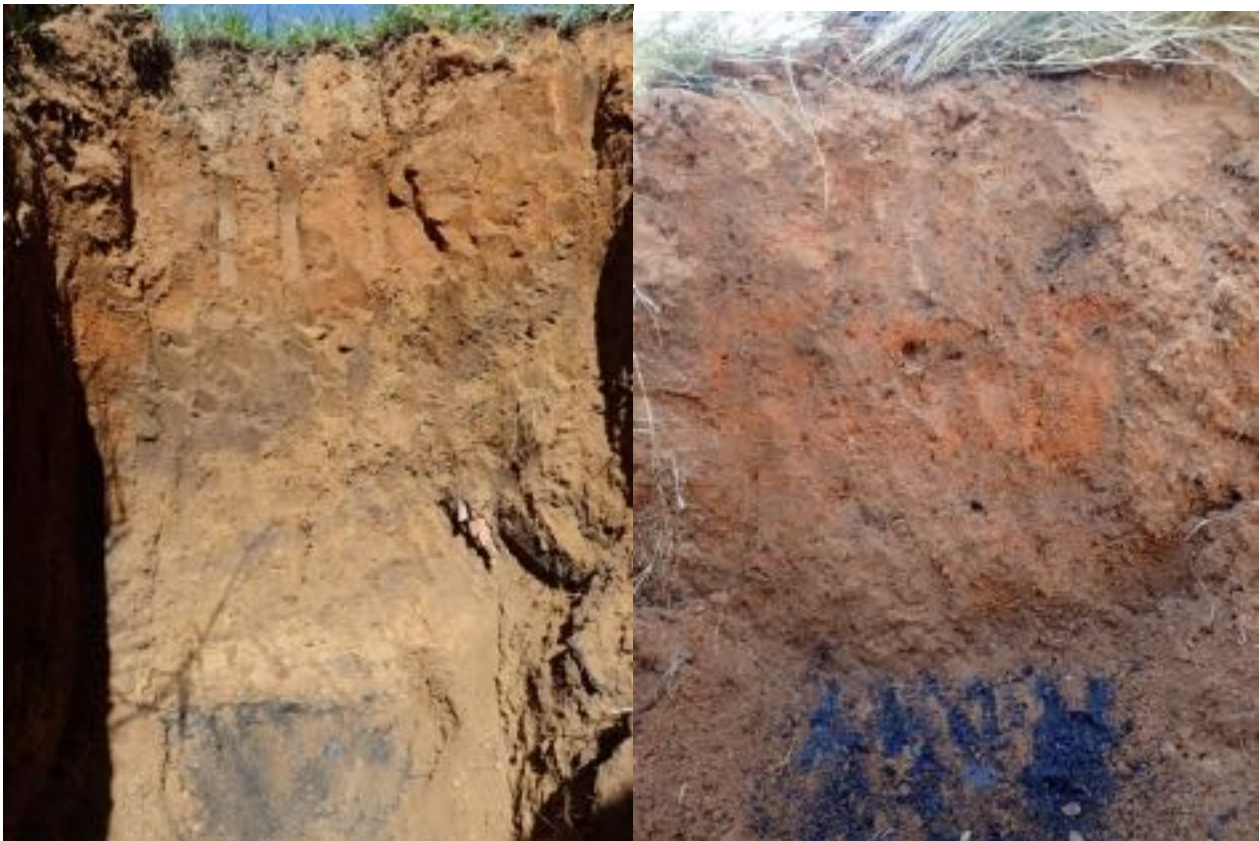
Figure set 63 Soils of the Witbank form with 170 cm and 60 cm soil depths to spoil respectively
