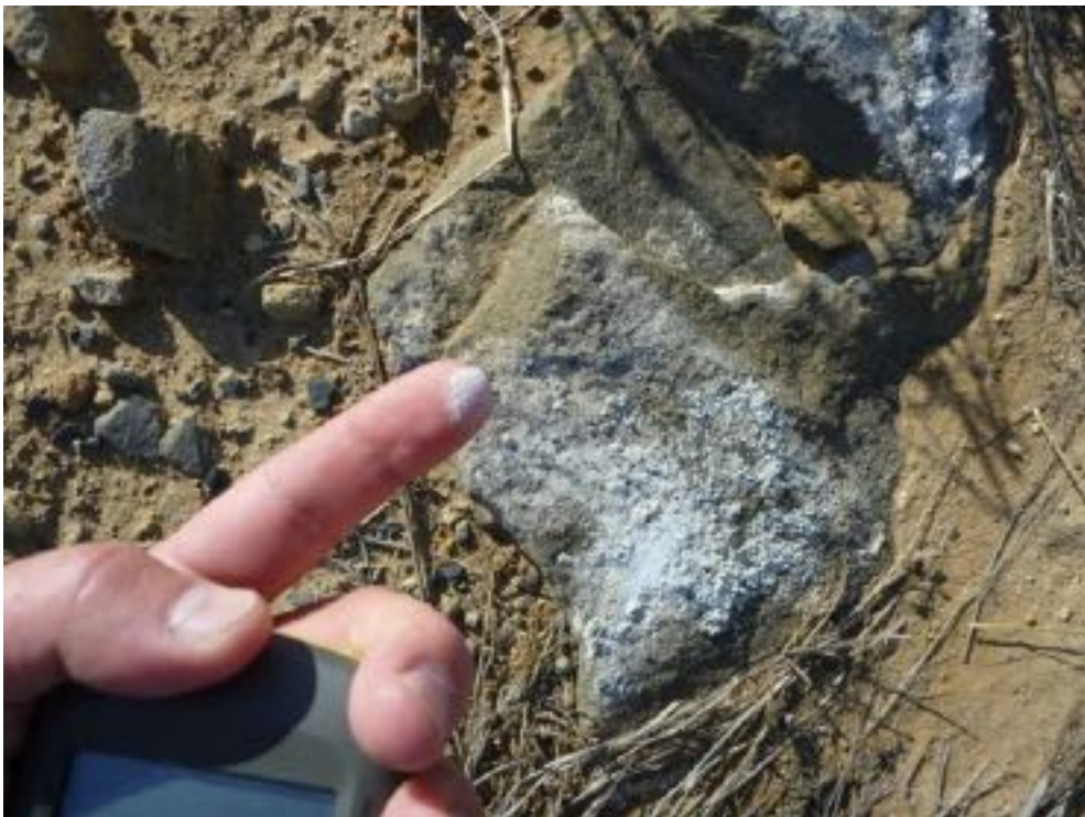
Figure 39 Sulfur salts on rock surfaces where pyritic materials have undergone oxidation
