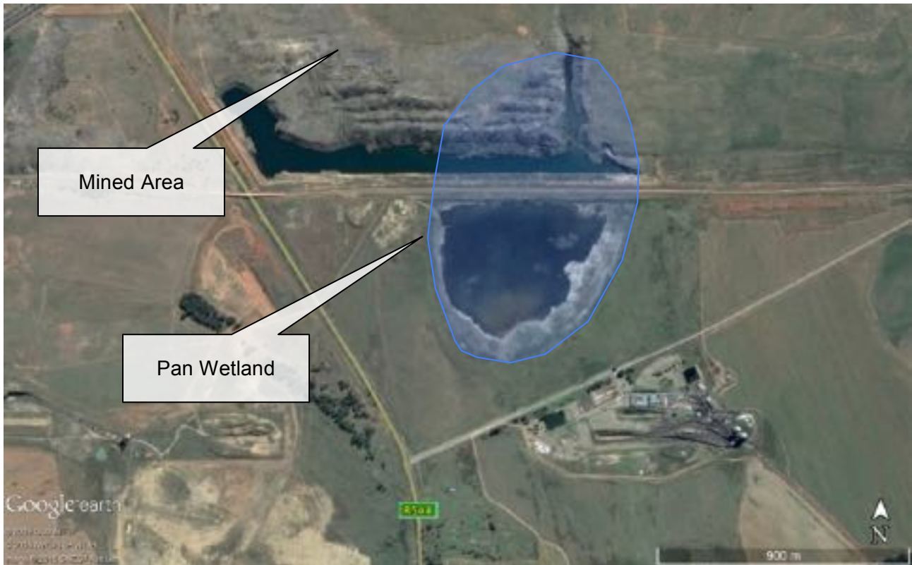
Figure 57 Inward draining pan system that has been cut in half
