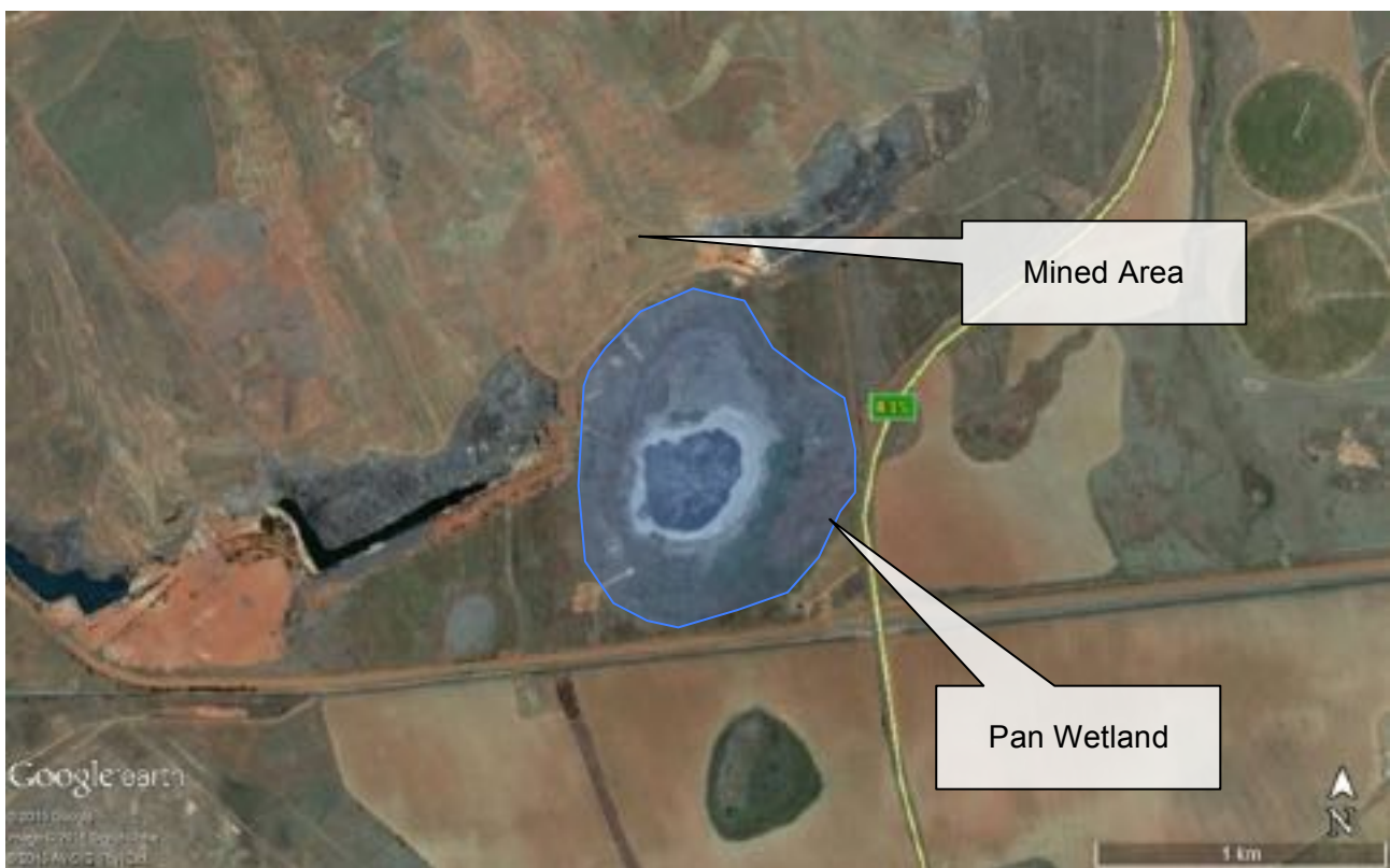
Figure 58 Inward draining pan system of which the catchment has been significantly reduced
