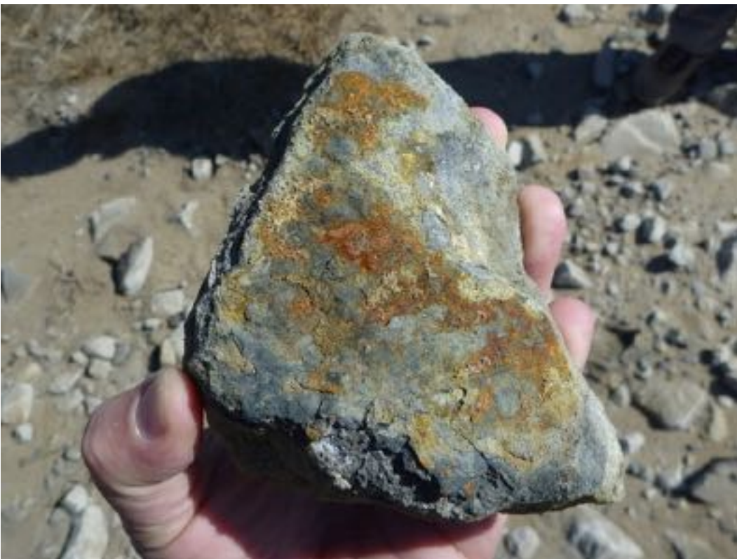
Figure 37 Pyritic sandstone rocks in the mined wetland area
